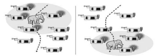
Fig.2.10 Detection of an event – an elephant that moves through the network along with the event source
