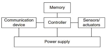
Figure 2.1 Overview of main sensor node hardware components
