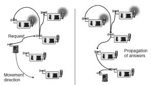
Figure 3.4 A mobile sink moves through a sensor network as information is being retrieved on its behalf
