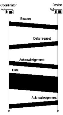
Handshake between coordinator and device when the device retrieves a packet
