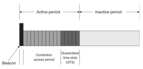
Figure 5.14 Superframe structure of IEEE 802.15.4
