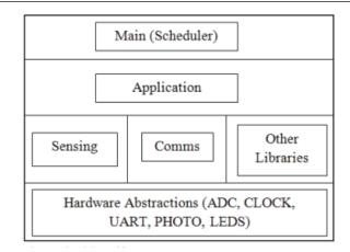
Figure 5.2 TinyOS Architecture
