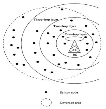
Figure: Layered architecture.
