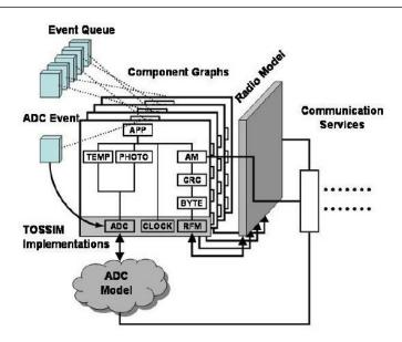
Figure 5.6 TOSSIM Architecture Source : Protocol and Architecture for Wireless Sensor Networks by Holger Karl , Andreas willig
