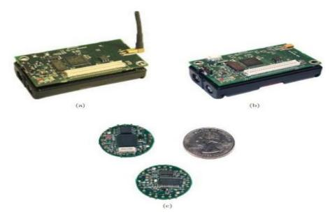
Figure 5.1 Berkeley Mote processor boards: (a) MicaZ, (b) Mica2, and (c) Mica2dot. Source : Protocol and Architecture for Wireless Sensor Networks by Holger Karl , Andreas willig
