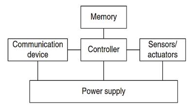
Figure 2.1 Overview of main sensor node hardware components
